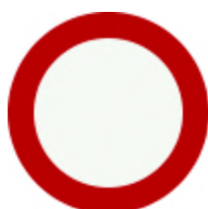
Road closed in both directions to vehicles, riders and persons in charge of animals or livestock
