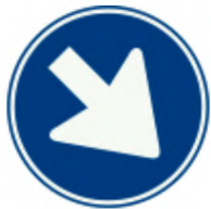
Instruction to all drivers to keep to the right of the sign (or left if arrow is reversed)
